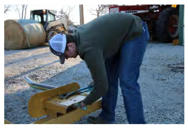
Ensuring my equipment is well-serviced before and during the wrapping season is key to efficiency and safety. Here, I'm adjusting the bale arm to accommodate different bale sizes, ensuring smooth operation when I arrive at a customer's field.
