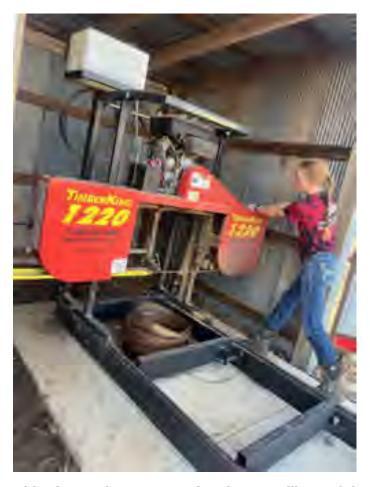
This picture shows me getting the sawmill out of the shed. You must check the sawmill over every time to make sure it is functioning properly and safely. The blade must be mentioned and checked for sharpness. It is very important to have a sharp blade as it is safer and makes cleaner cuts. You also must make sure that the water tank is full of water with a little soap added. The soapy water is used to lubricate the blade.
