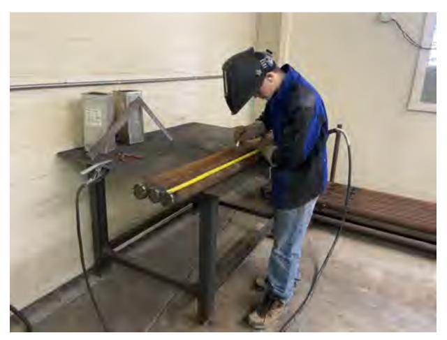
I'm carefully measuring my post to ensure proper placement before welding on my metal Orings. Taking accurate measurements is essential for achieving a precise and secure fit, preventing misalignment, and ensuring the rings function correctly. Proper placement also contributes to the overall strength and durability of the structure, reducing the risk of rework and ensuring a professional, high-quality result in the final build.
