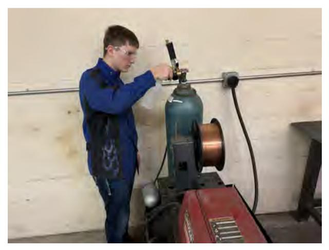
I'm carefully inspecting my valve gauge connection by spraying a soapy water solution on them to check for any air leaks. If there's a leak, bubbles will form, indicating a faulty seal or loose connection. This step is crucial for ensuring safety, preventing gas loss, and maintaining proper pressure for efficient operation. Regularly checking for leaks helps avoid potential hazards, improves equipment performance, and ensures a stable and reliable workflow in welding or gas-related applications.
