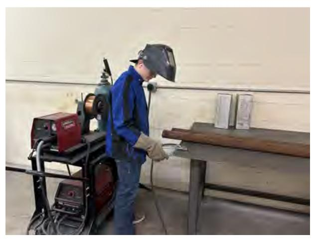
Here, I'm carefully inspecting the ground clamp to ensure it is securely attached and making a solid connection with the welding table. A proper ground is essential for maintaining stable arc performance, preventing fluctuations, and ensuring high-quality welds. Without a strong connection, you may experience issues like inconsistent arcs, excessive spatter, or weak welds. Taking the time to verify the ground setup helps improve efficiency, reduces defects, and enhances overall welding results.
