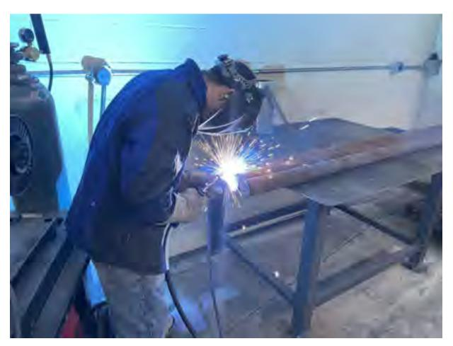
I'm welding caps onto the top of my fence posts to create a secure seal that prevents debris, water, and other contaminants from getting inside. This helps protect the interior from rust, corrosion, and structural weakening over time. By sealing the posts, I'm ensuring greater durability and longevity, reducing maintenance needs, and improving the overall strength and appearance of the fence for years to come.
